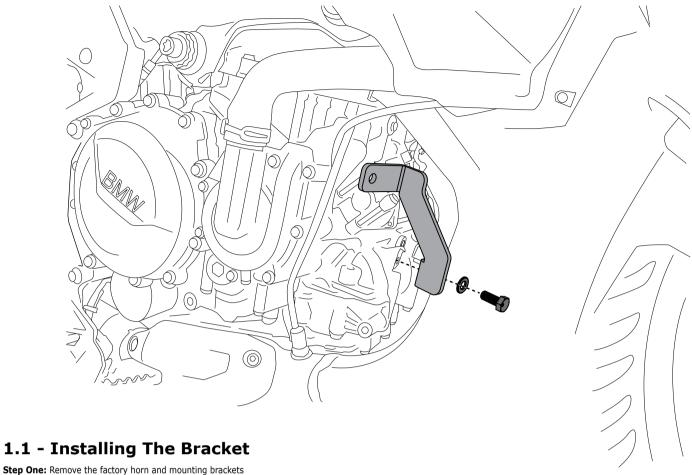
Step Two: Install the SoundBomb Mounting Bracket (a) to the factory horn mounting location using the supplied M8x20 bolt (b) and Washer (c).
