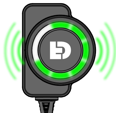
Flashing Green LEDs Light Circuit Two fuse setting mode
